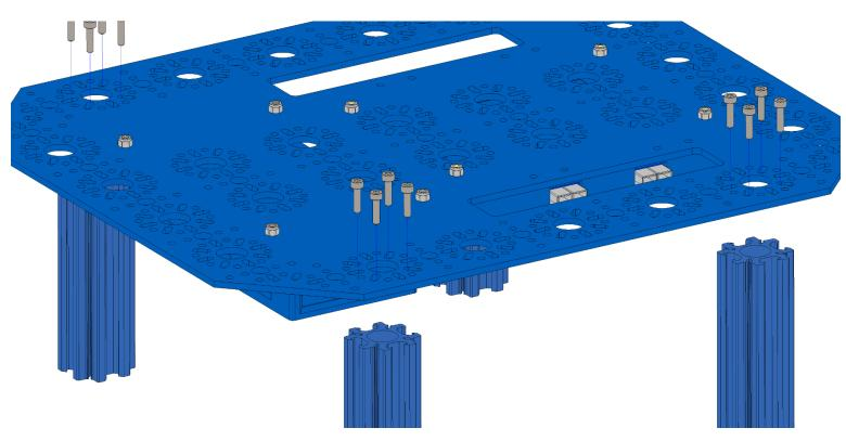
Attach one side of the baseplate to the existing T-slot extrusions with M3 x 12mm screws.
