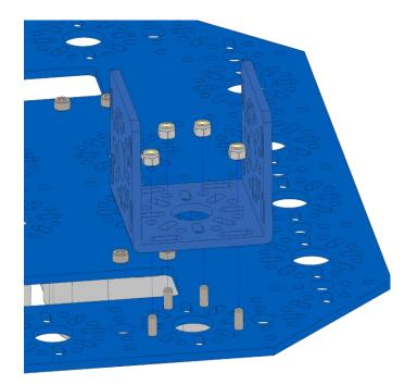
Attach the Maverick Motor to the motor mount plate using 6 M3 x 12mm screws.
