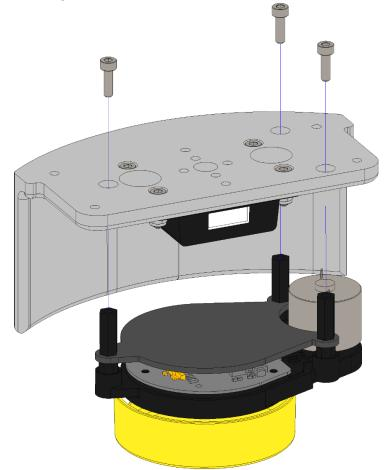
Attach the LIDAR mount to the baseplate using 4 M3 x 12mm screws and 4 M3 Nylock nuts.
