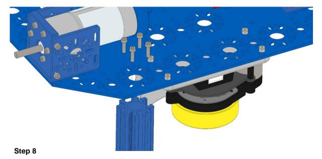
Insert a clamping hub V2 onto a motor shaft until the face of the shaft is a few millimeters from the face of the clamping hub. Tighten the 2 clamping screws.
