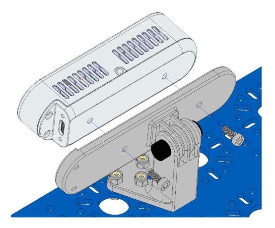
Using 4 M3 x 12mm screws, attach the other control panel mount to the other side of the base plate. Don't over tighten these screws.
