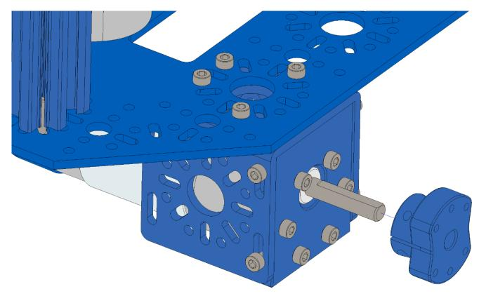
Insert an M3 x 25mm screw through the wheel and 3 plastic pattern spacers and screw it into the clamping hub. Repeat this step 5 times for the remaining screws. Repeat Step 8 for all the remaining wheels.
