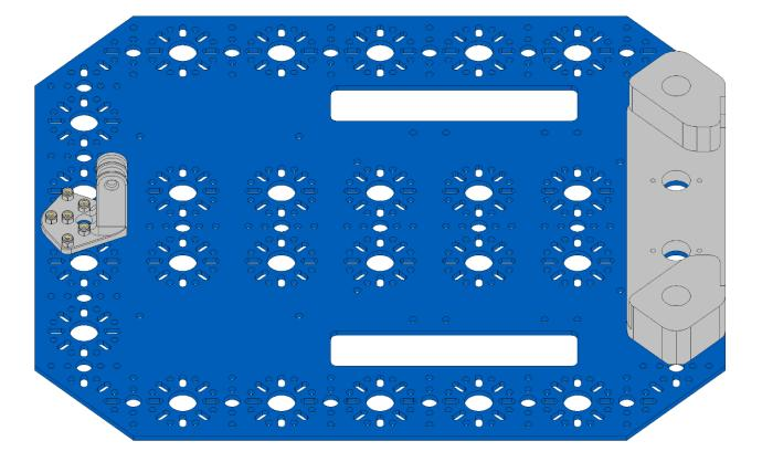
Using 2 M3 x 10mm screws, attach the control panel to the bottom mount on the robot. Don't over tighten these screws.
