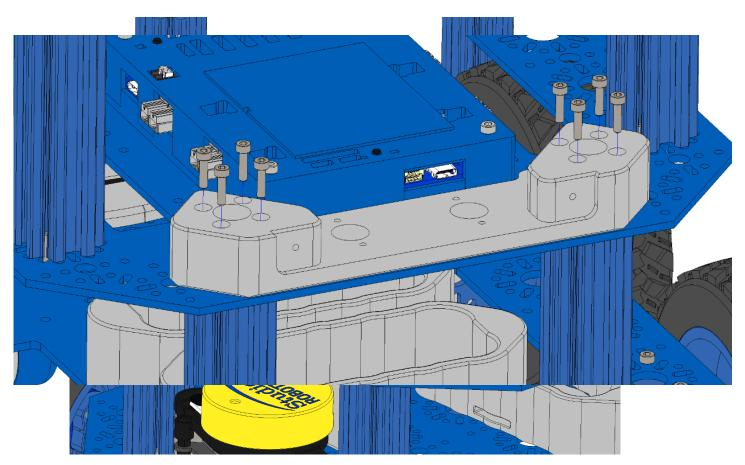
On the other side, put the screws through the control panel mount.
