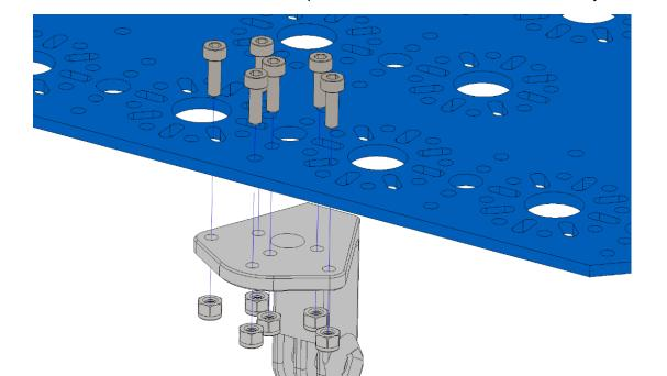
Attach the camera mount to the last base plate with M3 x 12mm screws and M3 Nylock nuts.
